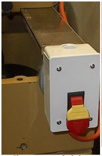
I've ... upgraded the switch and used a flat Carlon coverplate with a Grizzly switch #G8988.The coverplate and switch cost less than \$7 and now it looks like the "real thing".
