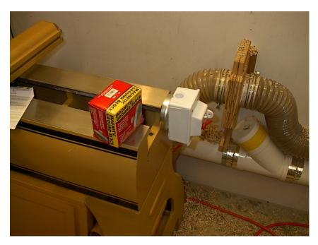
Remove the bolt and the two hex nuts from the magnetic ground block and use a hacksaw to cut ¼" off the length of the solid brass bolt. This will allow clearance for the switch after the block is mounted to the back of the box. Drill appropriately sized holes to fit the bolt and the wire you use to connect to the switch in the lathe headstock. Use only one hex nut to mount the magnetic block to the back of the box and tighten the nut as tight as possible.
