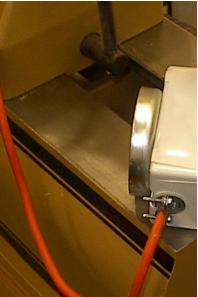
The magnetic unit is very powerful. I cut a donut from a piece of thick self adhesive vinyl and "stuck" it to the magnetic so now it can't even scratch the "Mustard Mistress".
