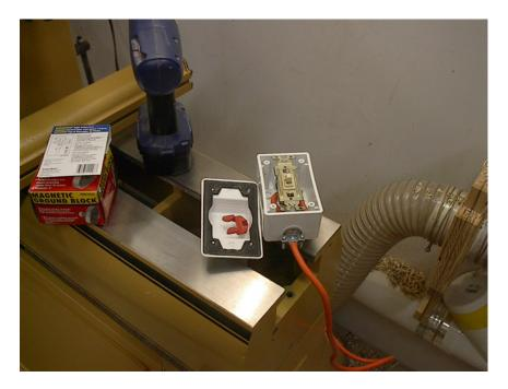
The switch is a simple 15 or 20 amp single pole light switch and sells from \$1.50 to \$3.50. A Magnetic Ground Block (used in welding applications) is available at most hardware stores and at Harbor Freight for \$3.50-\$5.00 depending on the current sale price. Total outlay should be less than \$20.00 and an hour of your "tinkering" time.
