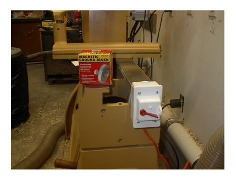
Screw a 3/8" electrical clamp connector for NM cable (part #20511) into the threads on the bottom of the box and tighten the two screws on the clamp to secure the wire to the box. (See first photo) 6-8 feet of wire should be enough. I used part of an old extension cord. Grounding is not required because you are simply wiring in the remote switch "before" the switch in the headstock. The headstock switch must be in the on position for the remote
